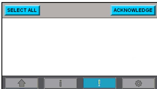
Figure 23 Alarm screen with no active alarms
