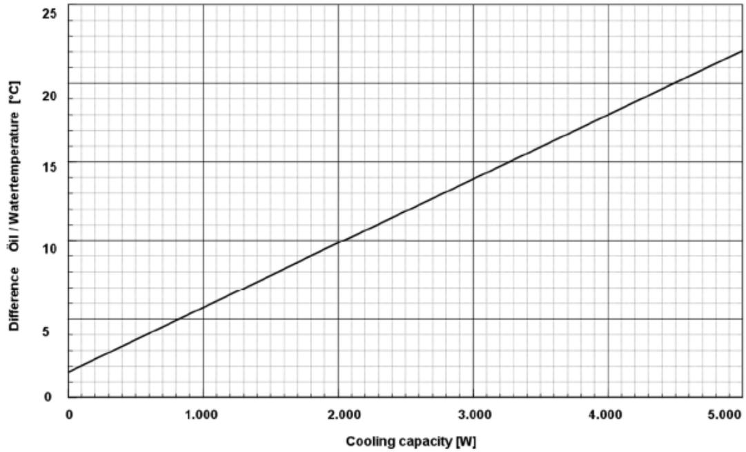
*Cooling capacity versus difference between entering water and supplied coolant temperatures*
