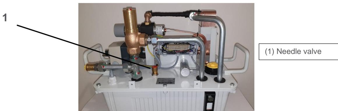
*Figure 7: Mounting position of the needle valve*
