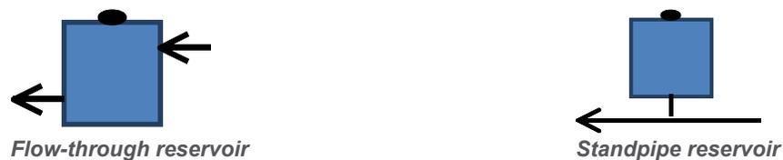
A standpipe reservoir introduces additional fluid to the liquid circuit as required, whereas a flow-through reservoir continuously exchange fluid. It is important to know that the pump simply needs to overcome the height and pressure difference one-time during start-up in a closed loop system, as the supply and return lines will equilibrate given that they have the same length and diameter.
