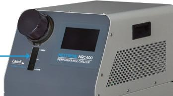
**While the unit is running, continuously add coolant to maintain the volume between the high and low marks. Ensure the coolant level stays within the specified range to avoid low coolant errors. If an error occurs, navigate to the error message and clear it.**
