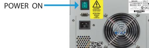
**Turn on the power switch on the back of the unit.**
