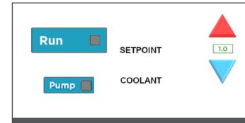
**Select the appropriate coolant, set point temperature and alarm values on the LCD. Refer to the user manual for complete instructions.**
