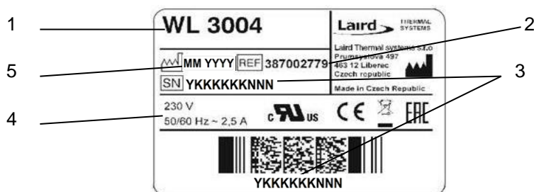
Fig. 2: Unit specific identification plate
