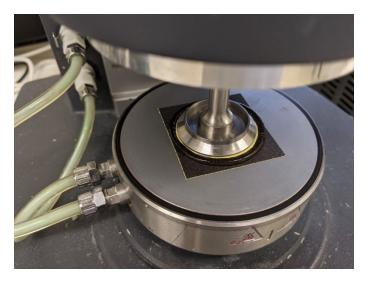
Parallel Plate Rheometer for liquids over a large temperature range
