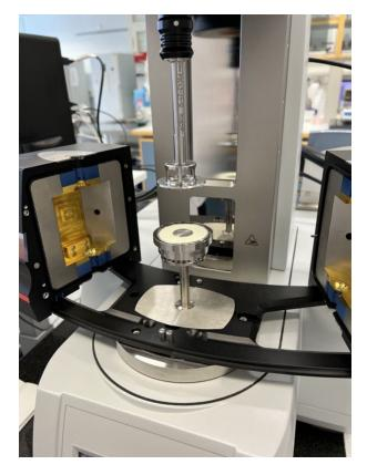
Rheometer for characterization of cell powder
