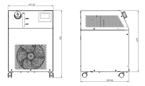
Figure 16 NRC2400 Chiller Overall Dimensions
