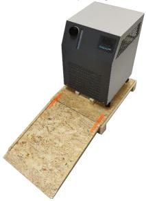
e) Then carefully and steadily roll the unit down the ramp. Care should be taken to make sure the unit does not roll off the side of the ramp.
