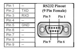
Terminal Settings: Baud Rate 115200, Data – 8-bit, Parity – none, Stop – 1 bit, Flow Control - none
