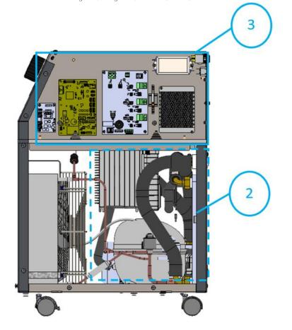
Figure 14 Coolant Circuit and Control Panel
