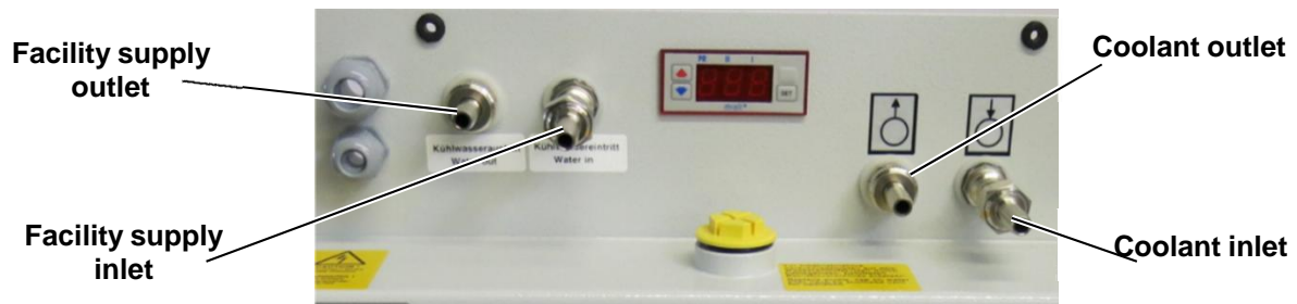
Fig. 8: Labelling of water inlet and water outlet
