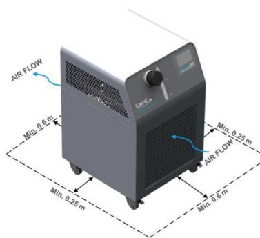
**Once the unit has been placed appropriately, lock the front casters. Follow all space requirements for installation.**
